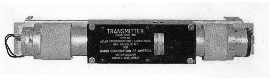
FIG. 9. View of the cavity oscillator or transmitter used in the "Walkie-Lookie" Pack Unit.
